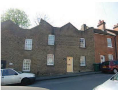
Picture 2.56 Nos. 1-4 Green Lane are unified by their angular parapet wall, also known as a Butterfly Roof
